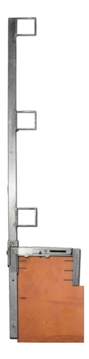
The Parapet Railing provides a 2x4 railing around the perimeter of a flat roof that has a parapet (curb) no greater than twelve inches wide (30 centimetres) when a platform is not required.
