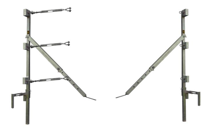
A Cable Railing can be used on the Parapet Bracket. The Telescopic Arm must be used on both ends where the cable connects to the Stanchion Post. The span between the ends can be no greater than thirty feet (9.1 meters) with two intermediate Parapet Brackets spanning no greater than 10 feet (3 meters) apart for a total of four Parapet Brackets every thirty feet (9.1 meters). The Telescopic Arm is not required for the intermediate Parapet Brackets. Turnbuckles are not included in the cost.
