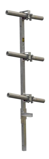
The Slab Rail provides railing around the perimeter of a concrete slab. The Tube and Clamp Railing can be used in all the Stanchion Post applications so the U Bolts are priced individually. The 1 1/2" pipe is also priced according to the the required length. The maximum span between brackets is ten feet (3 meters).
