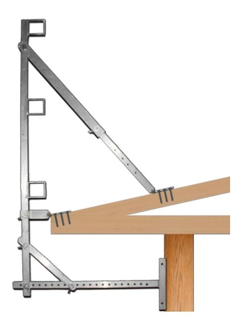
The Fascia Railing provides a railing at the edge of a roof when a platform is not required. It is connected to the roof at two points. This railing can be adjusted from a 4/12 pitch to a 12/12 pitched roof. The Right Angle Support Arm can also be adjusted to accommodate the various depths of a soffiit.
